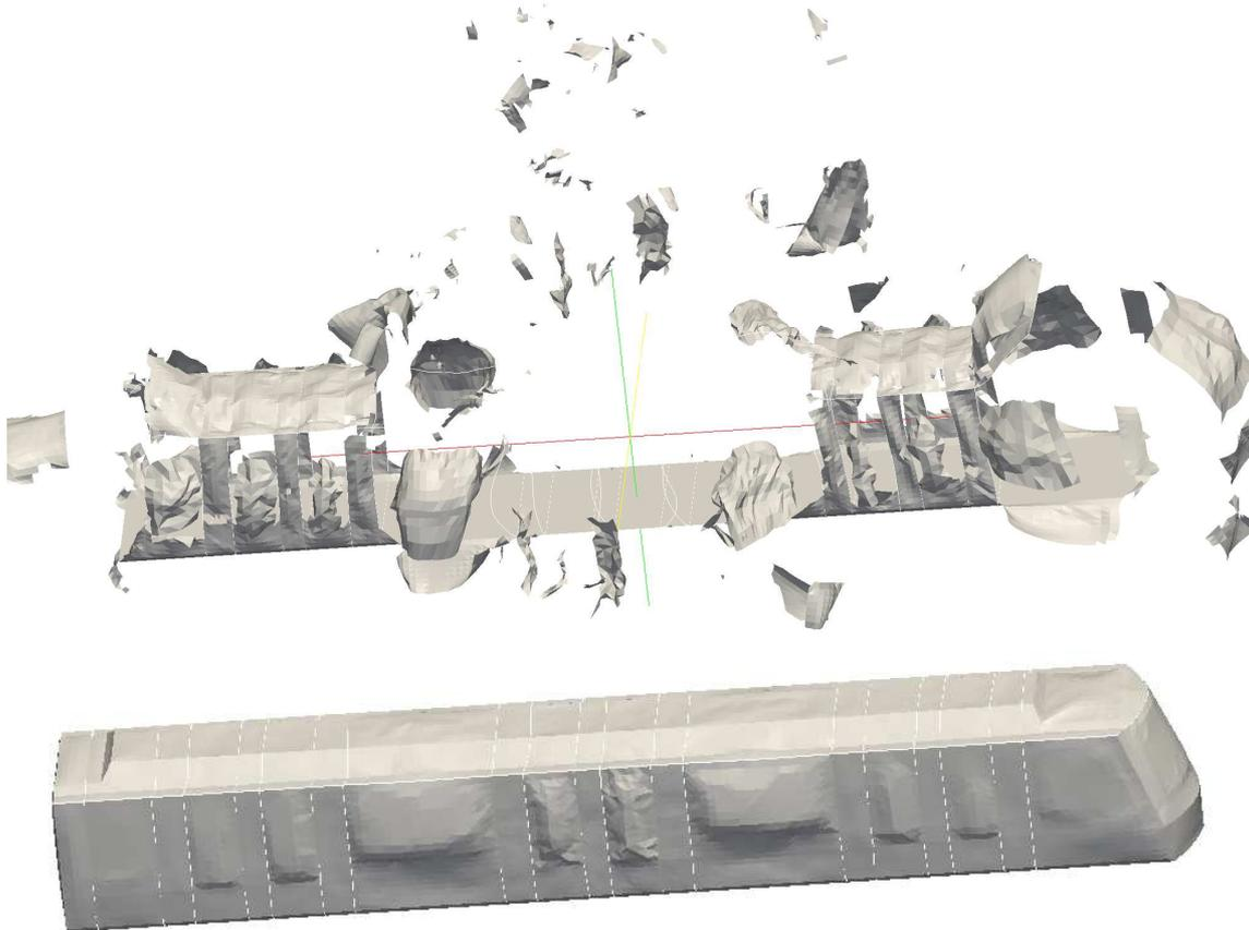
*Figure 5 Displacements after 6 ms for 10 kg TNT (top) and after 20 ms for 0.5 kg TNT (bottom), frame structure*
