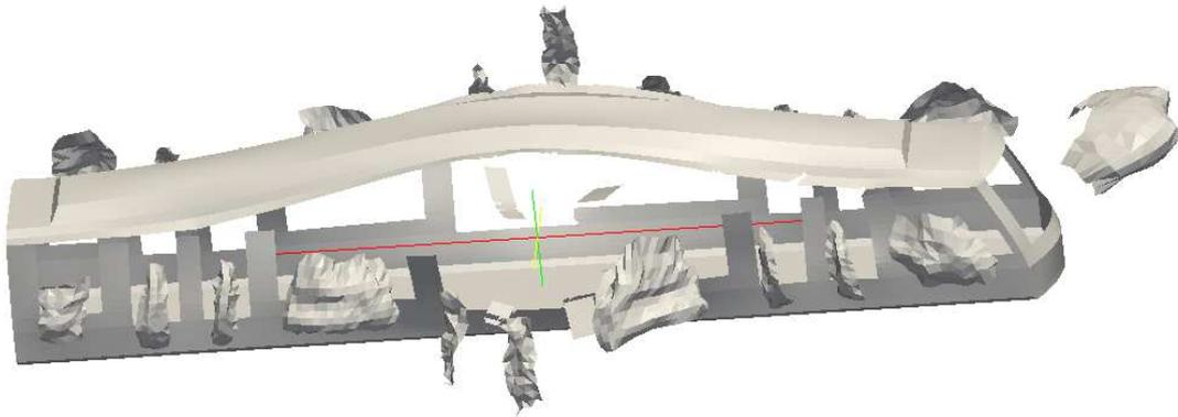
*Figure 6 Displacements after 20 ms for 10 kg TNT, sandwich structure*
