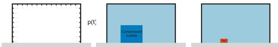
*Figure 3 Numerical models for air blast waves: pressure-time function, compressed balloon, solid TNT*
