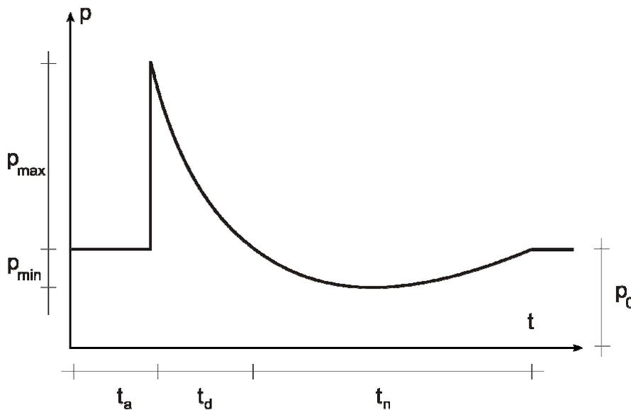
*Figure 2 Pressure history of an air blast wave*
