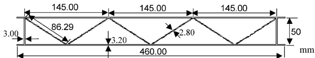
*Figure 4 Honeycomb structure for the train (see Zheng [9])*
